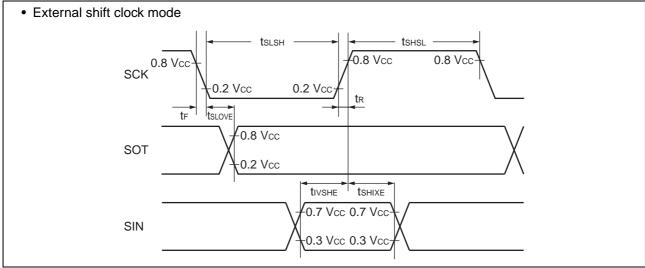
Sampling is executed at the falling edge of the sampling  $clock^{*1}$ , and serial clock delay is disabled\*<sup>2</sup>. (ESCR register : SCES bit = 1, ECCR register : SCDE bit = 0)
