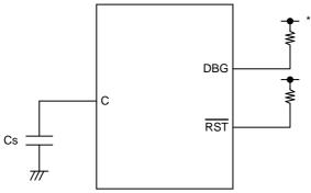
\*: Connect the DBG pin to an external pull-up resistor of  $2 \text{ k}\Omega$  or above. After power-on, ensure that the DBG pin does not stay at "L" level until the reset output is released. The DBG pin becomes a communication pin in debug mode. Since the actual pull-up resistance depends on the tool used and the interconnection length, refer to the tool document when selecting a pull-up resistor.
