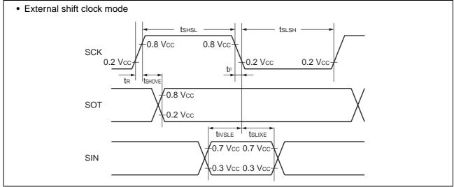
Sampling is executed at the rising edge of the sampling  $clock^{*1}$ , and serial clock delay is enabled\*<sup>2</sup>. (ESCR register : SCES bit = 0, ECCR register : SCDE bit = 1)
